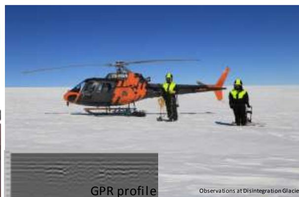
GPR observations on Disintegration glacier with snow cover as seen in GPR profile (inset).
